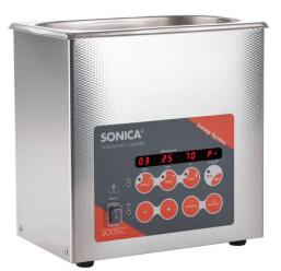
Stainless steel tank made in AISI 304 thickness 08/10 with round tank corners for a better removing of dirt residuals after cleaning process. The tank is conical and realized with a press machine
