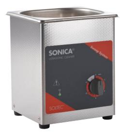
Stainless steel tank made in AISI 304 thickness 08/10 with round tank corners for a better removing of dirt residuals after cleaning process. The tank is conical and realized with a press machine
