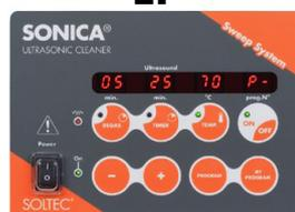
**Serie EP** The most technologically advanced of the SONICA range: **Sweep System** generator; modern digital display control panel windows; degas time setting; cleaning times from 0 to 99 minutes; tank liquid temperature setting up to 70°C; memory for 9 cleaning programmes; jet program function to start quickly and easily cleaning cycle.
