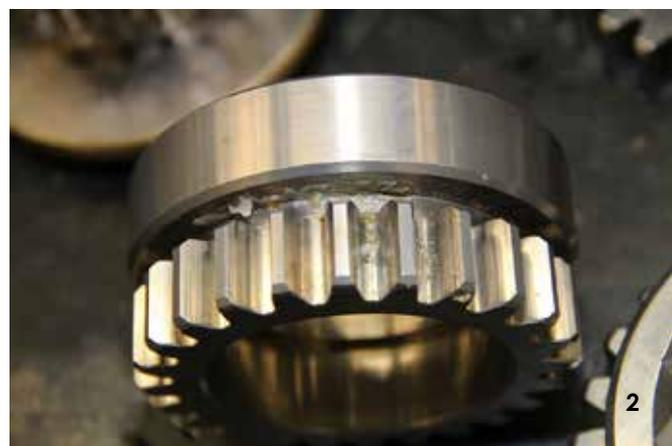
**Figure 1/2/4** - Details with obvious signs of dirt and oxidation before ultrasonic treatment
