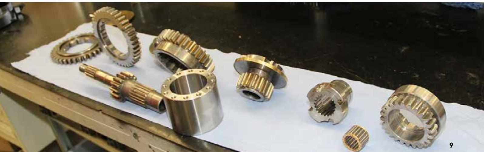
**Figure 9** - Various details after SONICA ultrasonic cleaning with SONICA ML concentrated alkaline detergent
