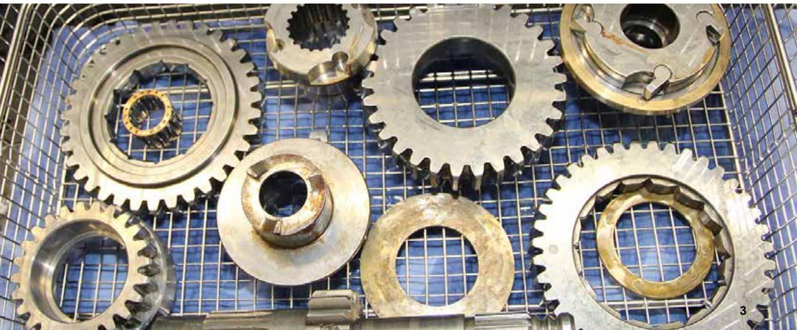
**Figure 3** - Winch parts before ultrasonic treatment
