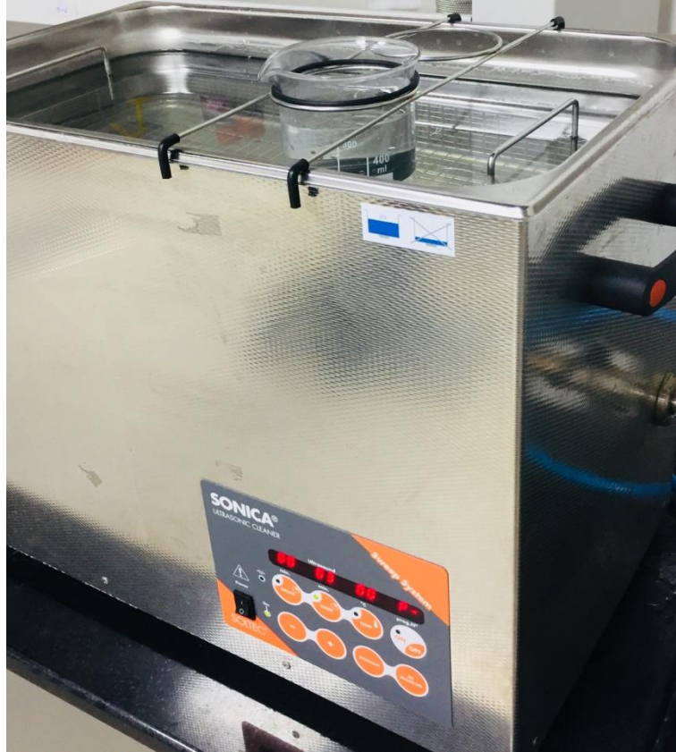
Figure 2. Top view of SONICA Ultrasonic Cleaner used for cleaning substrates at Nanostructures and Device Fabrication lab. IIT Indore, Madhya Pradesh, India.
