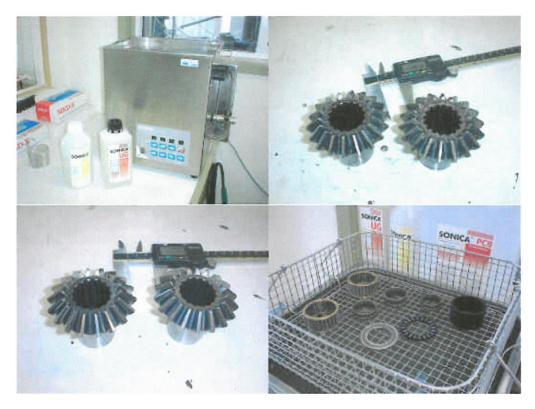
NDT or non-destructive testing forms an important part of our research & development process. Components selected for testing must be exceptionally clean and free from contamination. Ultrasonic cleaning is therefore a superior choice to ensure accurate results in dye penetrant testing.
